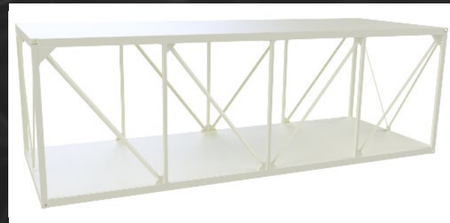
Bracing is installed to reduce dynamic stresses during transportation. The centre uprights are not required to support the roof structure once on site. Multi-level modules require a single centre upright for support.
